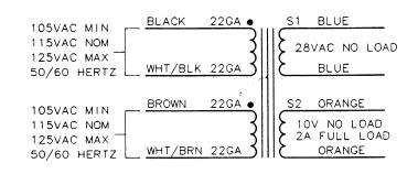
Note: Blue wires go to TB2, pins 1 & 2 on the driver.
